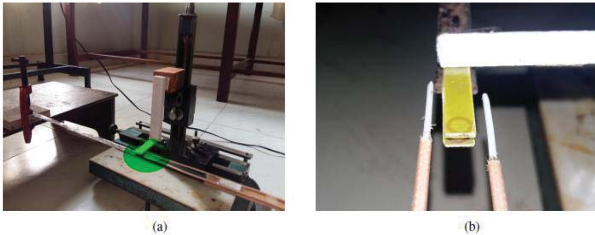
FIGURE 2. a) Photograph of a vibration sensor setup with cantilever and BCSRR system arranged between transmitting and receiving probes. b) Magnified view of BCSRR sensor probe.
