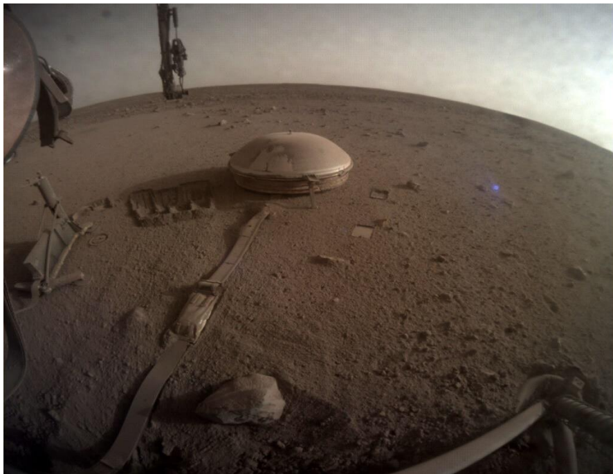
Figure 1.10: This is one of the last images ever taken by NASA's InSight Mars lander. Captured on Dec. 11, 2022, the 1,436th Martian day, or sol, of the mission, it shows InSight's seismometer on the Red Planet's surface. Image credits: NASA/JPL-Caltech.
