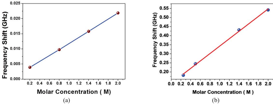
**FIGURE 3.** Calibration graphs obtained from the frequency shifts for (a) NaCl solution and (b) KCl solution
