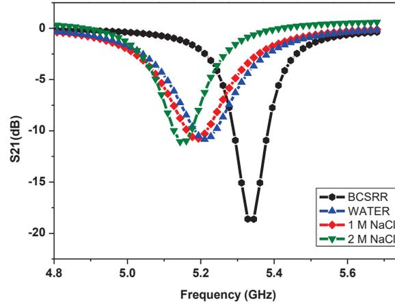
**FIGURE 2.** Transmission spectra corresponding to the BCSRR test setup with and without liquid samples
