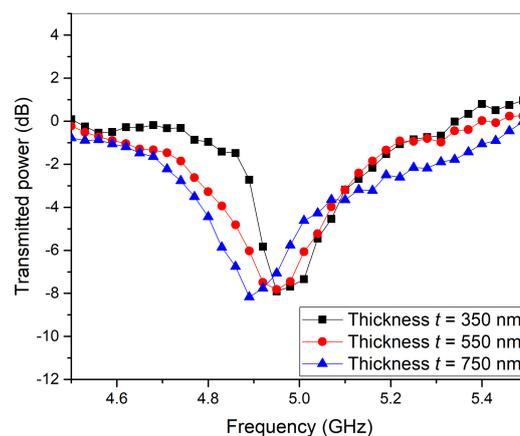
Fig. 2: Magnetic resonance in single square ring SRRs of different thicknesses  $t$  of 350 nm, 550 nm and 750 nm respectively made on glass substrate with dimensions - length  $l = 10 \text{ mm}$ , width  $w = 2 \text{ mm}$  and split width  $s = 1 \text{ mm}$ .
