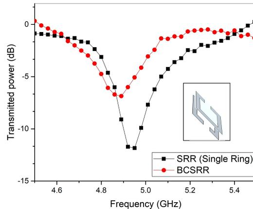
Fig. 3: Magnetic resonance in BCSRR of thickness  $t = 750$  nm made on glass substrate with dimensions length  $l = 10$  mm, width  $w = 2$  mm, split width  $s = 1$  mm and separation between rings  $d = 1.3$  mm along with the resonance curve for a single SRR with same values of  $l, w$  and  $s$ .
