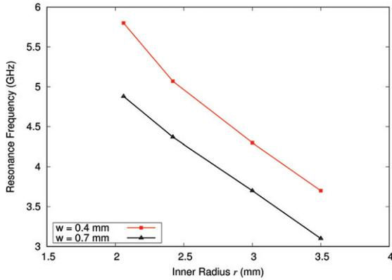
Fig. 6: (Colour online) Variation of resonance frequency of WSRR with inner radius  $r$  for two different wire diameters  $w$  keeping spacing between the rings  $s$  constant (0.97 mm).
