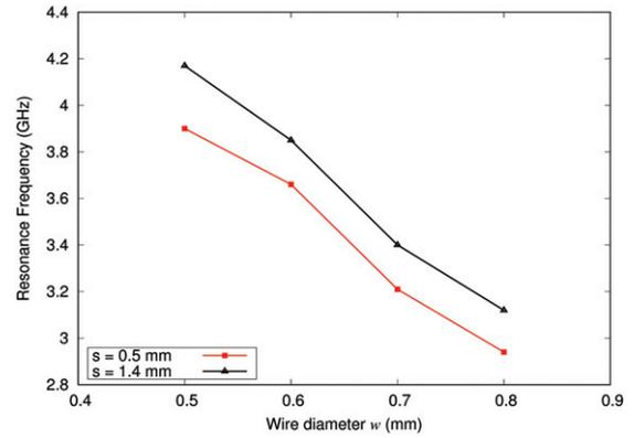
Fig. 8: (Colour online) Variation of resonance frequency of WSRR with wire diameter  $w$  for two different values of  $s$  keeping inner radius  $r$  constant (2.2 mm).
