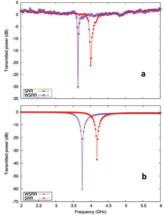
Fig. 4: (Colour online) Transmission spectra of Wire SRR (WSRR) and conventional SRR with the same structural parameters  $r$ ,  $s$ ,  $d$  and width  $w$  equal to the diameter of the wire: (a) experimental, (b) simulation.
