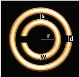
Fig. 1: (Colour online) Schematic representation of the proposed Wire Split Ring Resonator (WSRR) with structural parameters.
