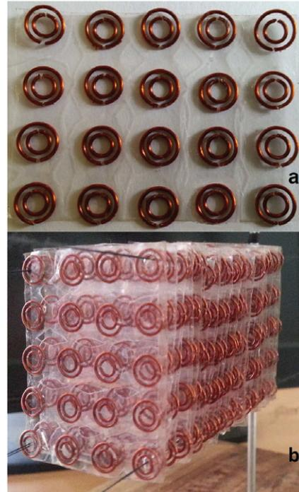
Fig. 2: (Colour online) Photograph of the WSRR constructed with structural parameters  $w = 0.4$  mm,  $r = 1.68$  mm,  $s = 0.5$  mm,  $d = 0.5$  mm. (a) Two dimensional array with periodicity of  $10$  mm  $\times$   $10$  mm; (b) bulk medium with periodicity of  $10$  mm  $\times$   $10$  mm  $\times$   $10$  mm.
