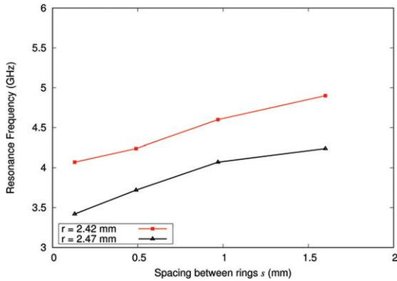
Fig. 7: (Colour online) Variation of resonance frequency of WSRR with the spacing between the rings  $s$  for two different inner radii  $r$  keeping wire diameter  $w$  constant (0.6 mm).
