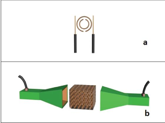
Fig. 3: (Colour online) Schematic representation of the experimental setup: (a) single WSRR between transmitting and receiving probes; (b) bulk WSRR medium placed between transmitting and receiving horn antennas.
