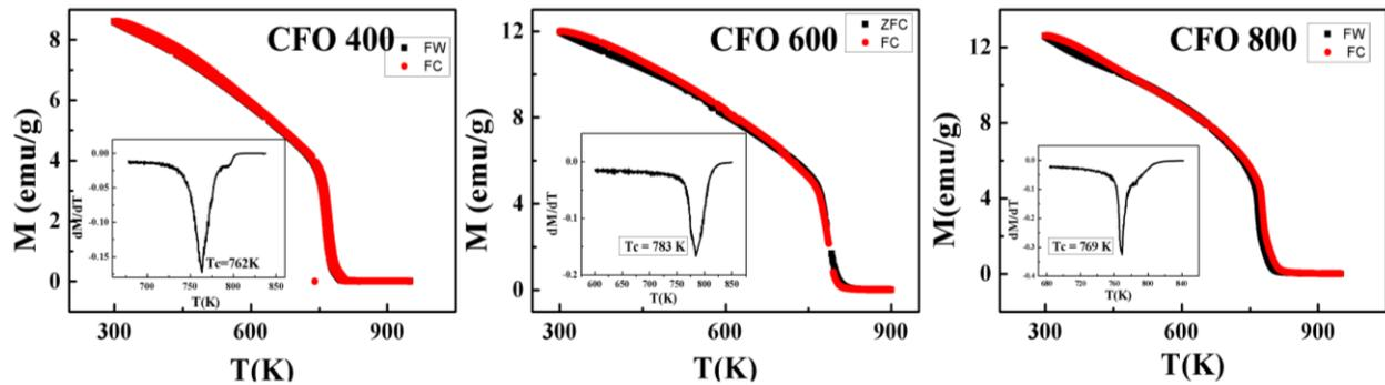
FIGURE 3. Temperature dependent magnetization  $M(T)$  of CFO 400, CFO 600 and CFO 800 sample.
