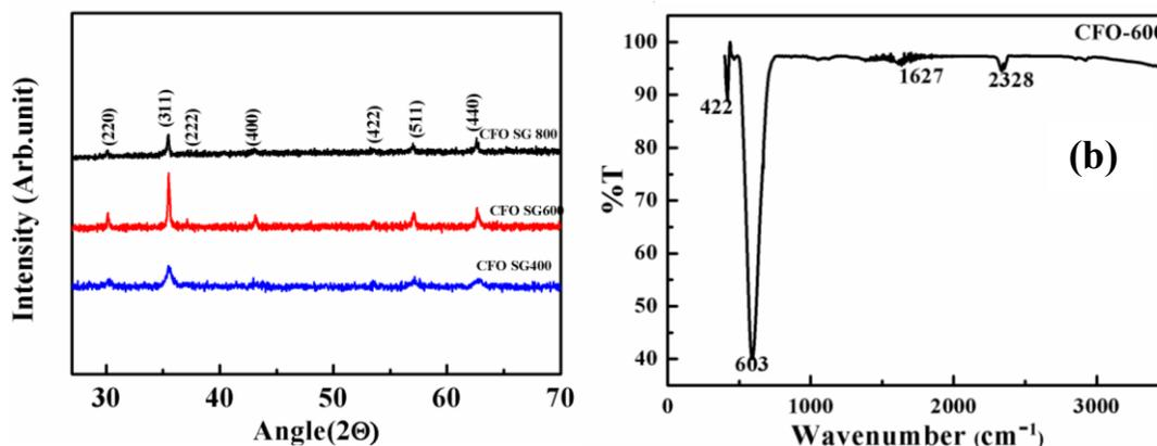
FIGURE 1 The X-ray diffraction pattern of CFO 400, CFO 600 and CFO 800 sample and FTIR image of SG 600 sample.
