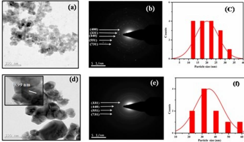
FIGURE 2 TEM images SAED pattern and particle size histogram of CFO 400 and CFO 600 sample.
