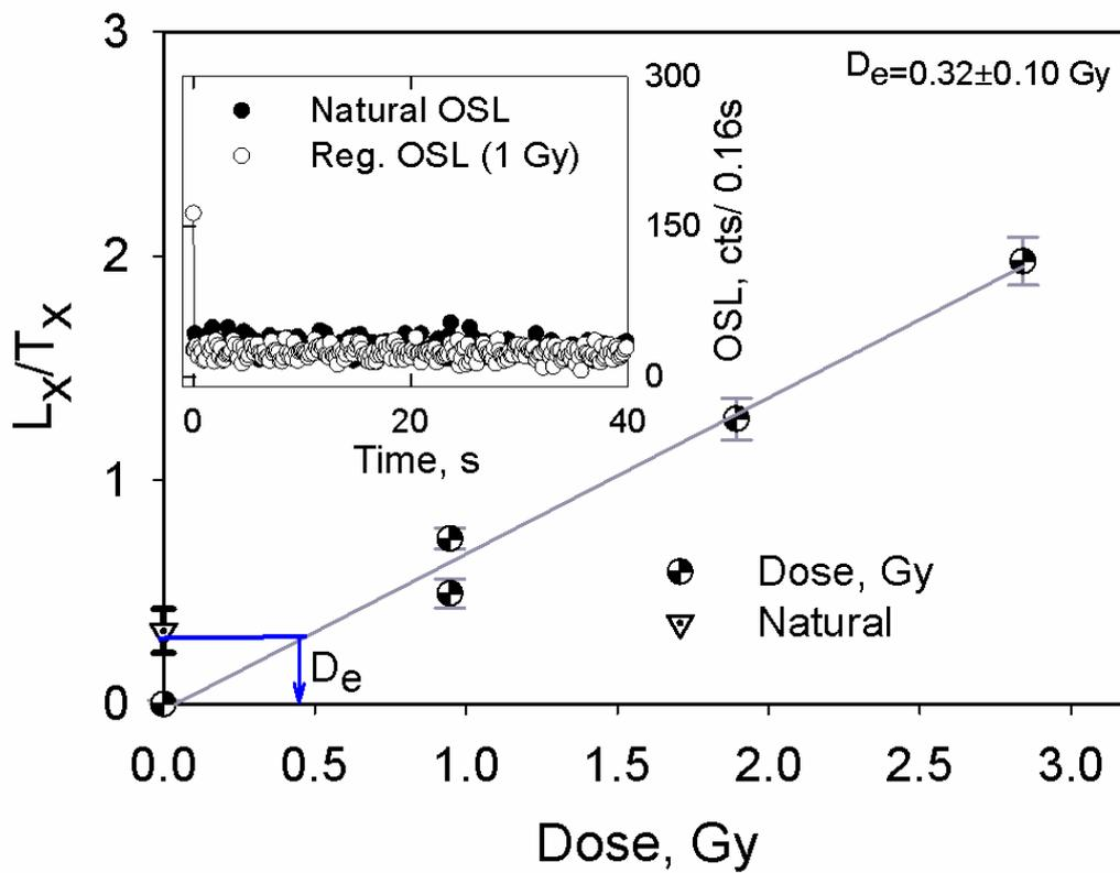
Figure 5. Diagrams showing the a) OSL growth curve of a representative sub-sample (ZAP-1), which had given a  $D_e$  value of  $0.32 \pm 0.10$  Gy. The inset figure shows the natural and regeneration dose decay curve of the same sample.
