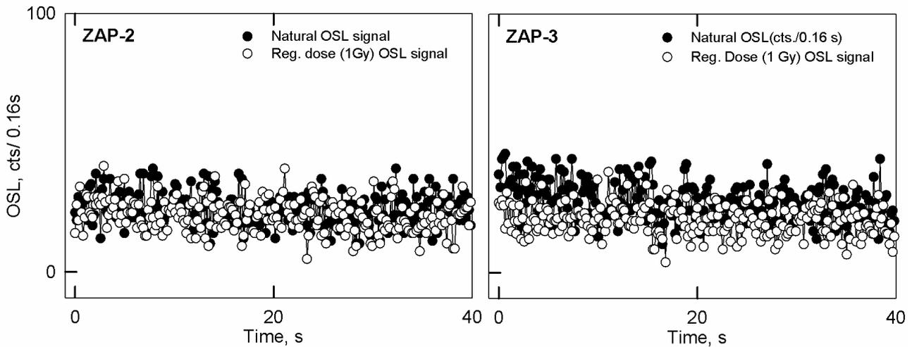
Figure 8. The OSL decay curve of samples ZAP-2 and ZAP-3 showing poor noise to signal ratio for both natural and regeneration dose. The figure also shows the insensitivity of the sample to the regeneration dose of 1 Gy (compare with the acceptable signal for ZAP-1, inset of Fig.5).
