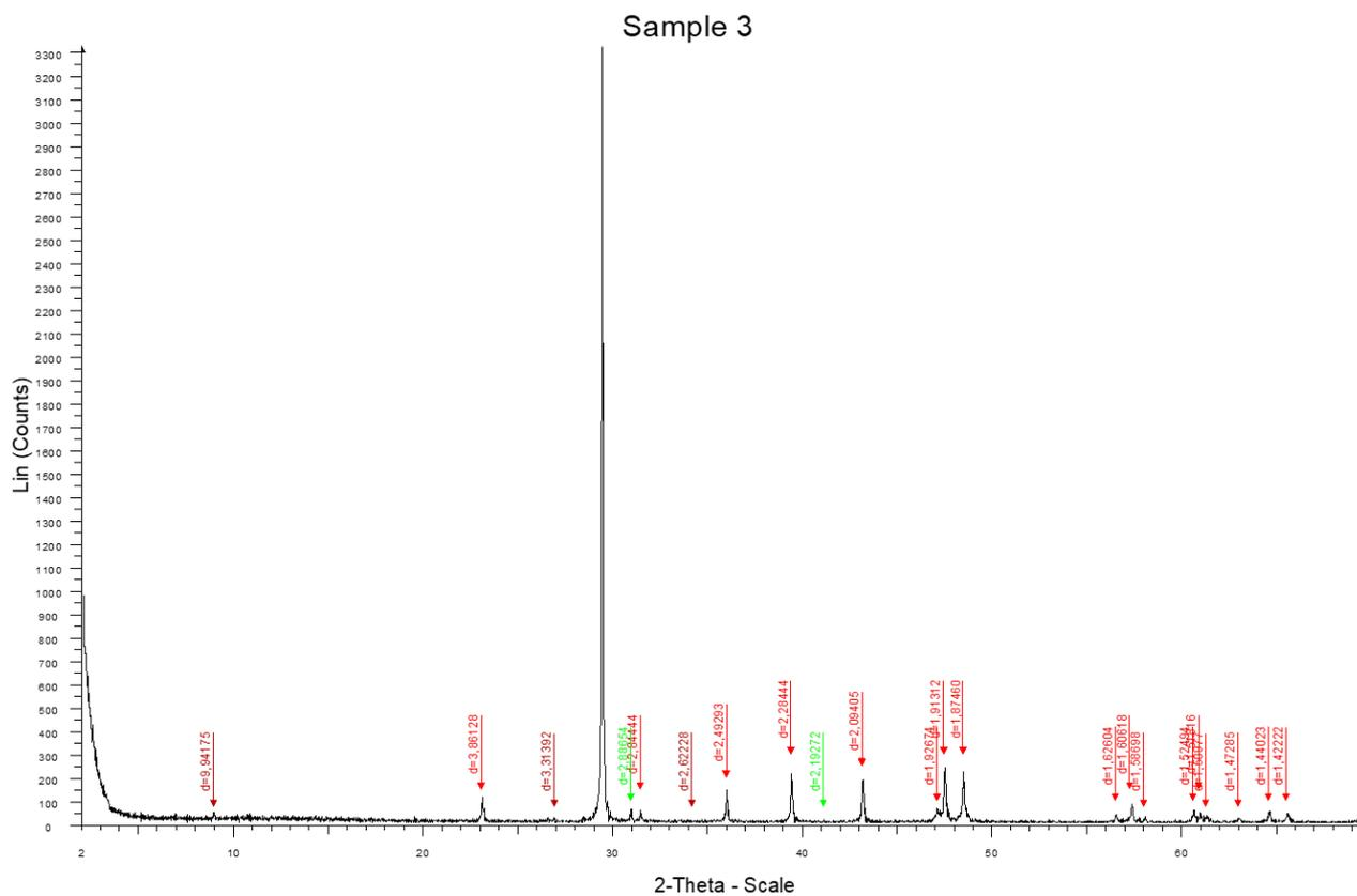
Figure 3. Typical XRD spectrum for ZAP1, 2, 3. ZAP1: with predominate of calcite (red), and traces of quartz (blue), dolomite (green), ZAP2: calcite (red), quartz (blue), dolomite (green), ZAP3: calcite (red), dolomite (green), biotite (brown).
