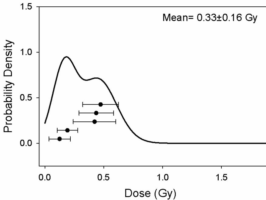
Fig.7 De distribution of sample ZAP-1 with mean value of accepted aliquots are shown. Twelve aliquots were measured for their OSL and five have passed the acceptance criteria and provided a mean equivalent dose of  $0.33 \pm 0.16$  Gy.
