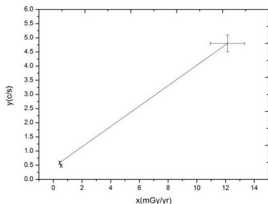
**Figure 4.** Linear relationship of counts versus dose rate of the radioactive pads, and floor at control room (0.48c/s).
