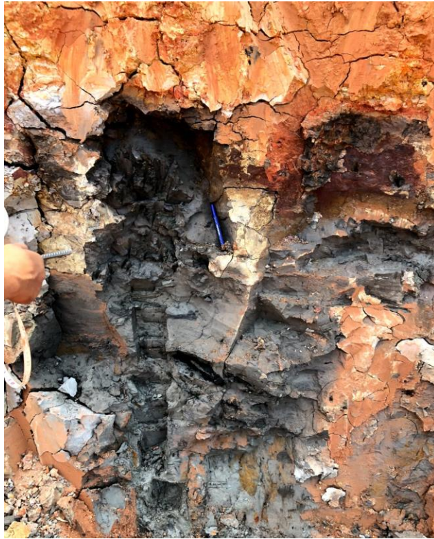
Fig - 2 shale samples taken in 10cm interval
