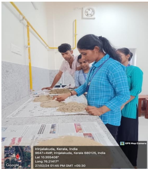
Fig.7 Cone and quartering method
