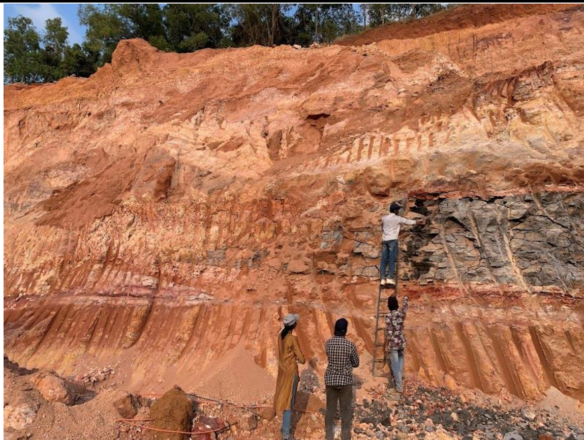
Fig -12 samples taken in 10cm interval.
