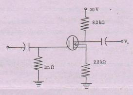
If  $ID_{SS} = 8mA$ , Vp = -8V Determine  $I_{DQ}$  and  $V_{GSQ}$  and  $V_D$  (Q is operating point)
